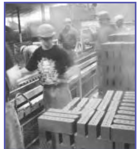
Bricks are cut by machine and stacked by hand, ready to go to the kiln
